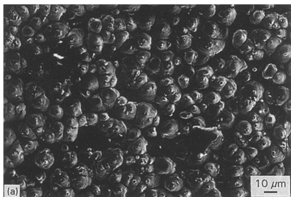
Figure 3 Scanning electron micrograph of a top view of laser-grown films on SiC.
